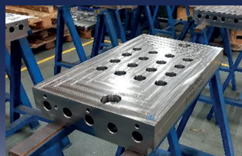
Heat Platens Material FerryNox 52 (finish machined, with thru boring)
