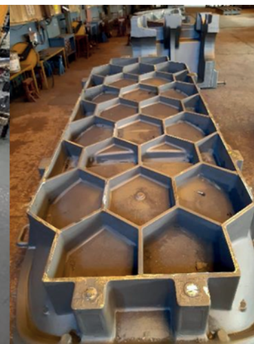
Helicopter lower shell mold with integrated ribs, Ferrynox N36 equivalent to Invar 36
