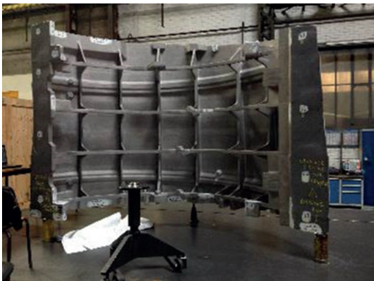
Acoustic tool A350 Hollowed-back designs: mass reduction with structural integrity
