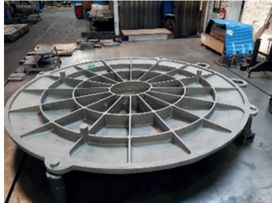
Satellite Invar mold one-piece tooling. No welded parts: better homogeneity, less deformation
