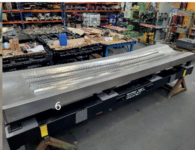
Caul plates tooling with improved rigidity design (max single piece casting length is 12 m)
