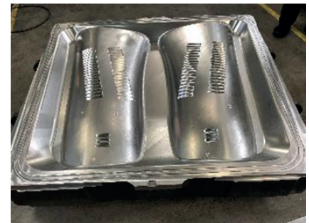
Heat Exchanger SPF tool A320 Ferrynox 52
